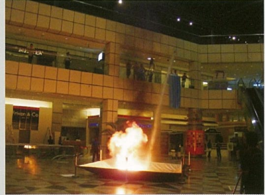
LIVE FIRE/DISCHARGE TEST OF EKOOL ZSS-25A WATER MONITOR AT SUNTEC CITY MALL
